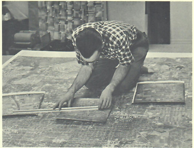
County, city governments use aerial mosaics extensively in planning. Largest one-piece mosaic obtainable is 8-feet wide, 12-feet long
