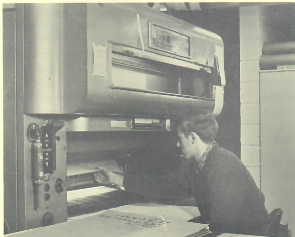
Over 60,000 prints, from 12 x 18 to 34 x 34 inches, are reproduced yearly on Ozalid Printmaster.
